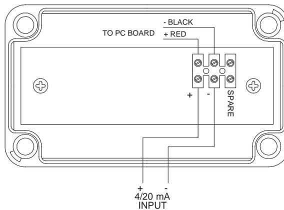
**Fig. 5 Field Wiring**
