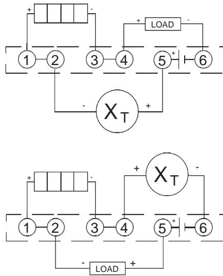
Fig. 2 Typical Wiring For 2-Wire Field Transmitter
